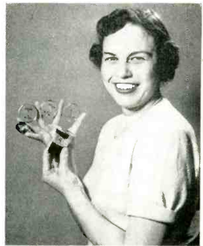
Example of slices cut from plastic-filled tube without disturbing positions of delicate grid wires
