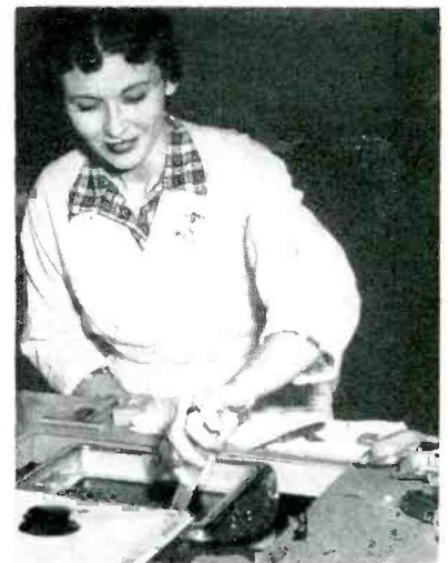
Dipping matrix in liquid plastic to form mold to be used for potting
