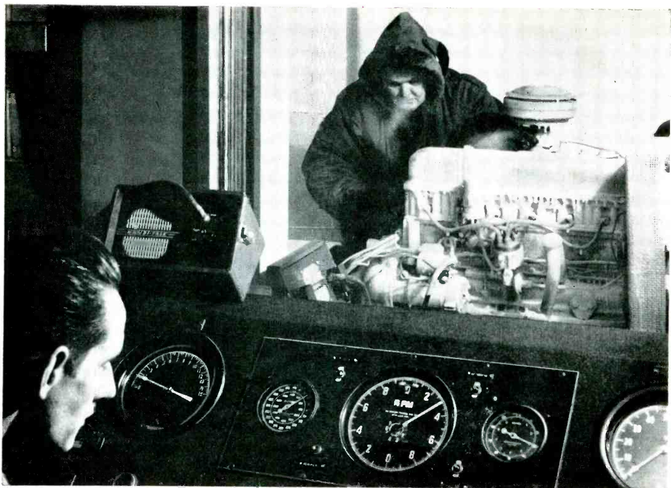
Standard Chrono-Tach shown front and center in "deep freeze" engine testing laboratory. (Courtesy of Thompson Products, Inc.)
