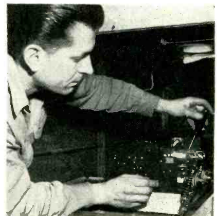
Installing a gyro servo unit in fuselage after removing rear panel of baggage compartment. Cables run from sprocket chains to aileron and rudder controls
