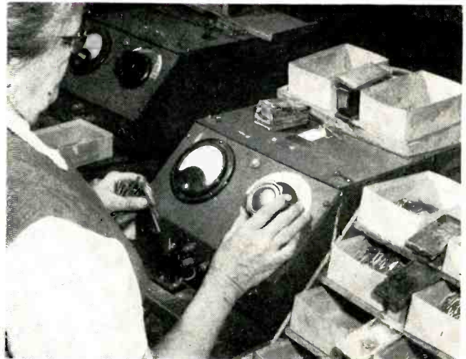
Core checker, with one core in position in vertical test coil mounted on a bench in front of QX checker. The four pads between the boxes on the stand at the right each hold a different color of paint for coding the ends of the cores
