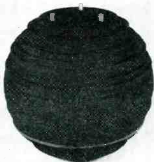
FIG. 4—Spherical Luneberg lens before (left) and after (right) foam binder application
