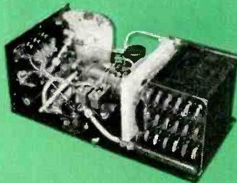
MODEL MB-177, TYPE 202 DISSIPATION: 1,700 watts. ALTITUDE RANGE: sea level to 50,000 feet. POWER REQUIRED: 110 volt, 400 cycle, 3 phase. WEIGHT: 27 pounds. SIZE: 10" x 19 15/32" x 7 3/4" high, per JAN-C-1720A, size B1-D1.
