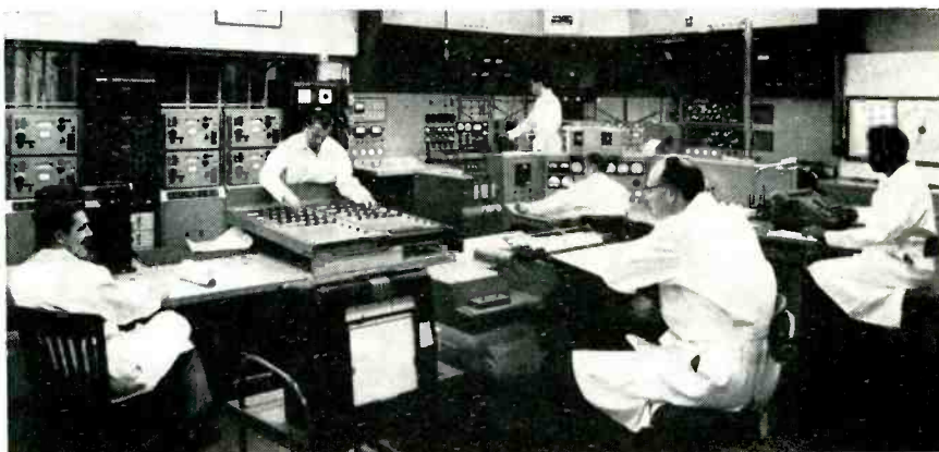
Control of models in the Southern California Cooperative Wind Tunnel at Pasadena is carried out in this room. At the potentiometer read-out cabinets (left rear) electrical impulses are converted into numbered figures. Data applicable to final design is obtained in a matter of seconds from the adjacent electronic computing center. The tunnel is operated by California Institute of Technology.
