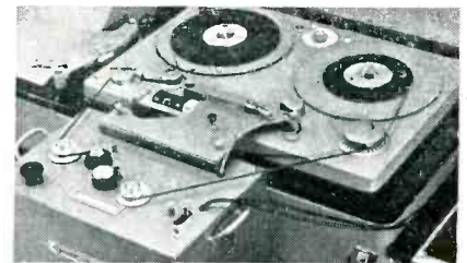
Acoustic time regulator manufactured by Telefonbau and Normalzeit attached to magnetic tape recorder
