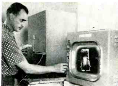
Display like that of home television screen is used to give brighter picture and protect personnel in industrial x-ray inspection
