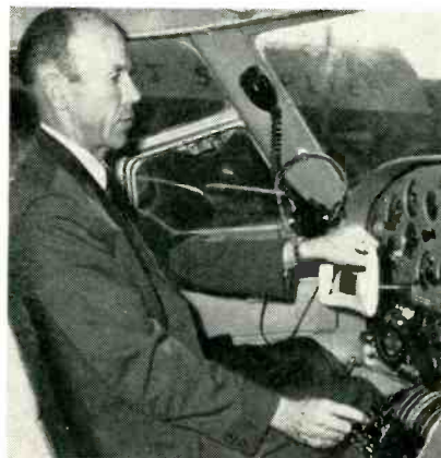
Autopilot control box mounts on control pedestal of twin-engine Cessna. Pilot is demonstrating adjustment of trim control at left of turn and pitch controls
