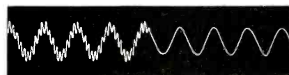
Oscillograph of sine wave, without (left) and with (right) compensation signal subtracted.
