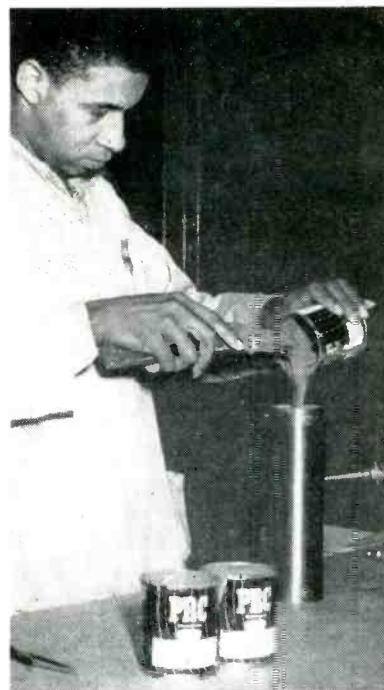
Loading injection gun with rubber compound in preparation for potting
