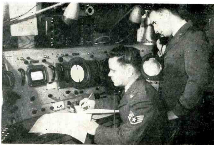
FIG. 1—Air Force personnel man Blue Hill 3.2-cm radar around the clock. Control boxes for automatic cameras are above main scope and scope camera assembly is at right
